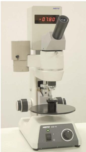
**Figure 2:** A radiuscope in the determination of the BOZR of an RGP contact lens. The microscope is focused on the lens surface, where an image of the spoke pattern can be seen, and the scale is set to zero. The microscope is focused on the aerial image of the spoke pattern, and the BOZR of the lens is retrieved. The depicted lens has a BOZR of 7.80 mm.
