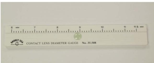
**Figure 13:** A V-shaped measuring gauge (V-gauge) with an appropriately positioned RGP contact lens for its total diameter determination. The depicted lens has a total diameter of 8.9 mm.
