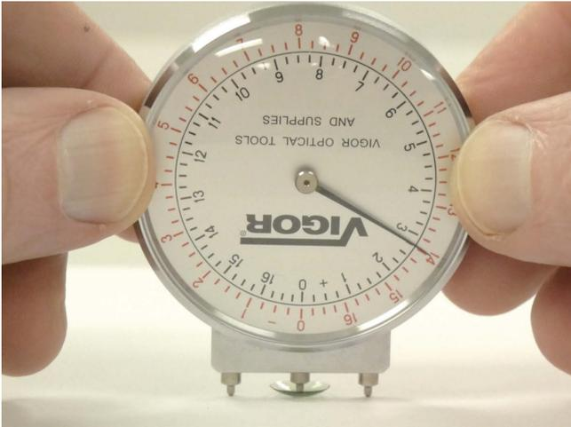
**Figure 23:** A lens clock while measuring the center thickness of an RGP contact lens. With its convex surface down, the dry lens is placed on a flat surface. One diopter on the black power scale equals 0.1 mm thickness. The depicted lens has a center thickness of 0.275 mm.
