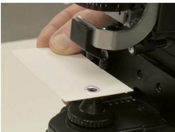
**Figure 18:** A paper card with a punched hole, used as a small lens stop for determining RGP lens back vertex power with a lensmeter.
