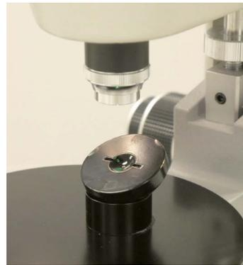
**Figure 6:** The lens mount is tilted when using a radiuscope to check the mid-peripheral back surface radii of an orthokeratology lens. These radii constitute a zone in orthokeratology lenses that is supposed to align with the wearer's mid-peripheral cornea.
