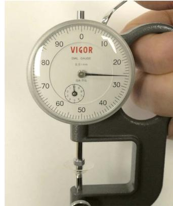
**Figure 20:** A thickness gauge (mechanical micro-meter) while measuring the center thickness of a scleral lens. The depicted lens has a center thickness of 0.26 mm.
