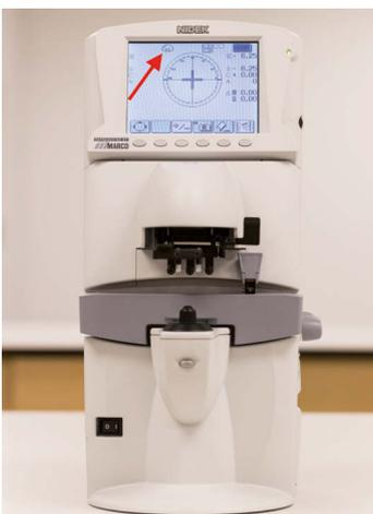
**Figure 19:** Electronic lensmeter with a contact lens measuring holder during the power verification of an RGP contact lens. The contact lens measurement mode is displayed on the screen.
