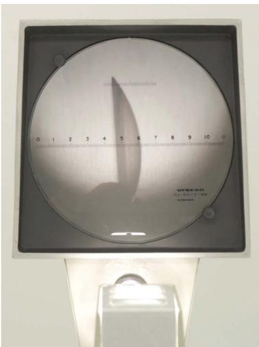
**Figure 25:** Inspection of the edge profile and the edge thickness of an RGP contact lens with a projection magnifier.
