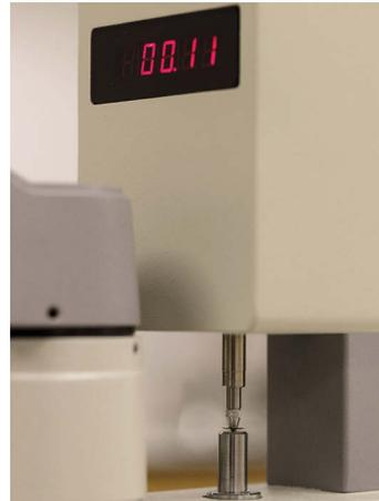
**Figure 21:** Determination of the center thickness of an RGP contact lens using the integrated thickness gauge of a radiuscope. The lens is positioned with its convex surface down. The displayed measurement value corresponds to the actual center thickness. The depicted lens has a center thickness of 0.11 mm.
