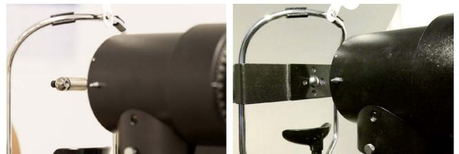
**Figure 7:** Different variants of lens holders for verifying the BOZR of a rigid contact lens, attached to the headrest of a keratometer. During measurement, the contact lens front surface rests on a drop of saline in the lens holder's concave depression.
