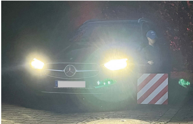
Figure 3: Exemplary representation of the veiling luminance induced by car headlights: The reduction of contrast due to stray-light becomes visible.
